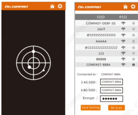
2.4、 Reconnect the phone to access the Internet. Password is the password of upper router. The SSID will add "-2G/5G" of the upper router SSID.
